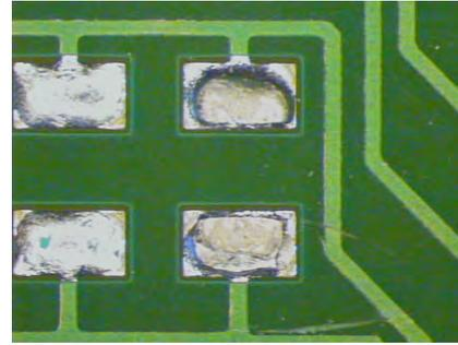
**Figure 7, cleaned without US,                      cleaned with US**
