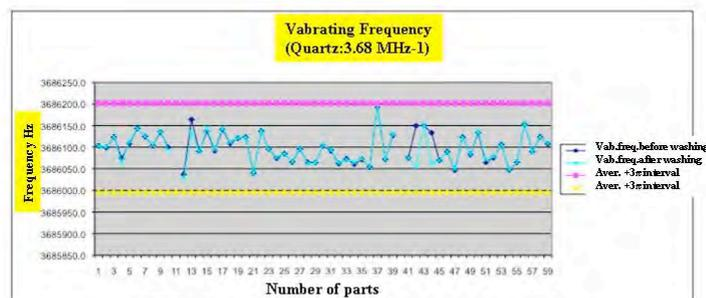
Figure 6: Quartz cleaned with ultrasonics. No damage
