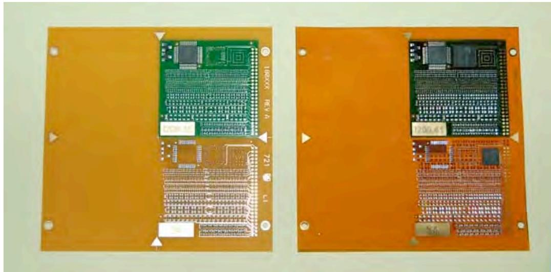
**Figure 3 : PCBs for trials, rigid and flexible**
